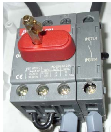
Figure 15: DC switch with four contacts tested in operation at Fraunhofer ISE. Three contacts are connected in series for one pole, one contact switches the second pole.
